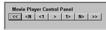
Figure 3. A movie player control panel used to step through an algorithm’s evolutionary search path. Here the user can jump back to the first generation (<< generation 0), step back N generations (< N), step back one generation (< 1), play forward through the evolution a generation at a time (>), step forward one generation (1 >), step forward N generations (N >), or jump forward to the final generation (>>).
