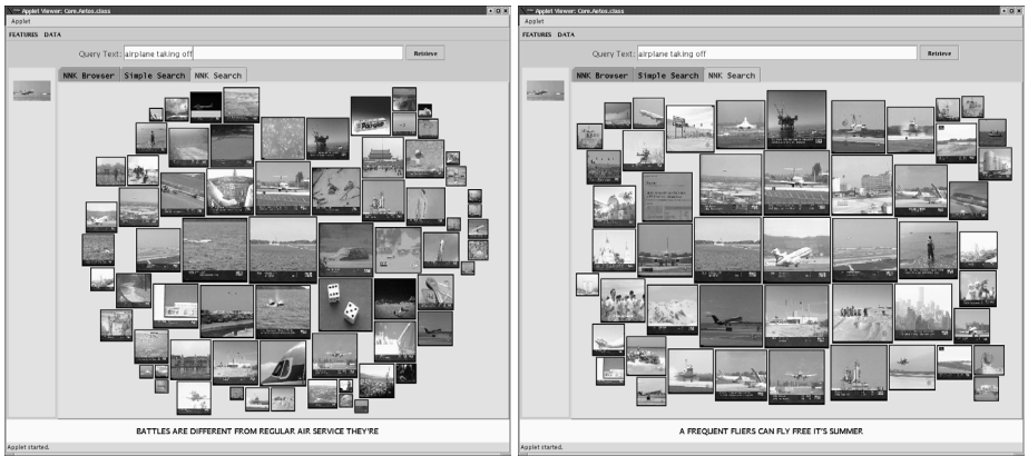
Fig. 3. The display of the first and second step of the NN^k search. The left figure displays the NN^k for the query images shown on the left canvas (planes taking off). The size of each image is proportional to the number of weights for which it was ranked top. The image north-west of the center has been selected as a relevant. The right canvas shows the improved results obtained when querying with the weight set associated with the selected image. See text for details.
